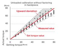
Surgic Pro calibration ensures outstanding safety because it minimizes deviations and ensures virtually no upward variations from pre-set values. As the graphs show, no calibration can be accurate without taking handpiece usage conditions into consideration.
